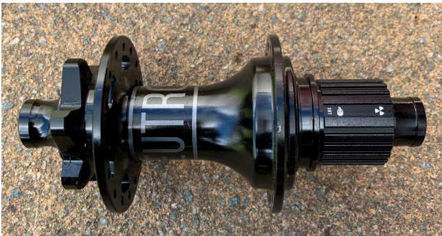
26. Apply the dust cover for the bearing
