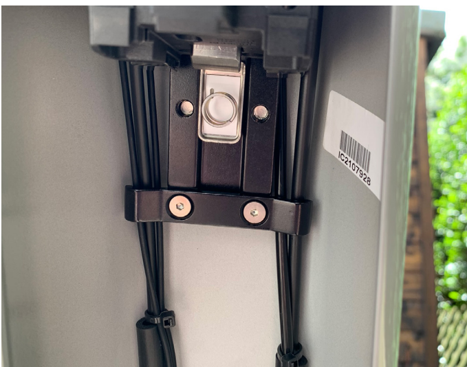
15. Put the battery mount back into the frame and loosely insert bolts
