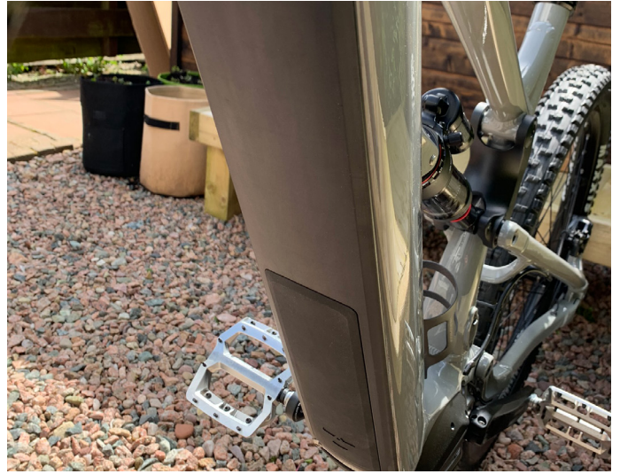
18. Refit battery door by sliding over the two bolts and tightening then reinsert the top bolt and tighten
