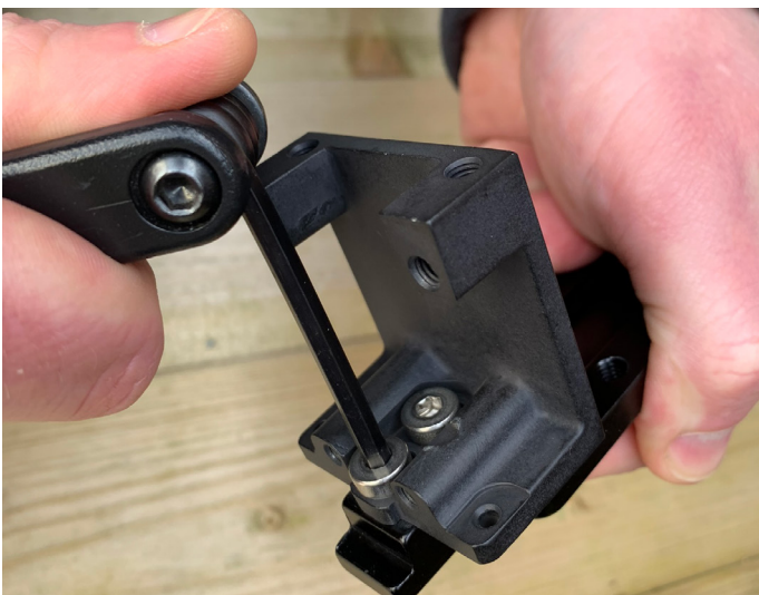
9. Undo the two bolts holding the mount to the back plate
