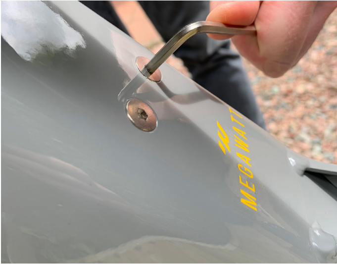
5. Remove the two bolts which hold the battery mount in place at the top of the downtube
