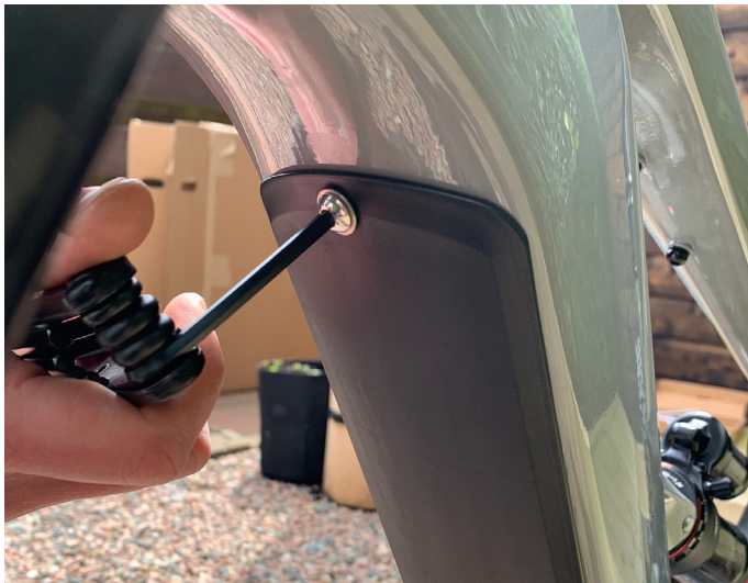
1. Remove the top bolt on your battery door
