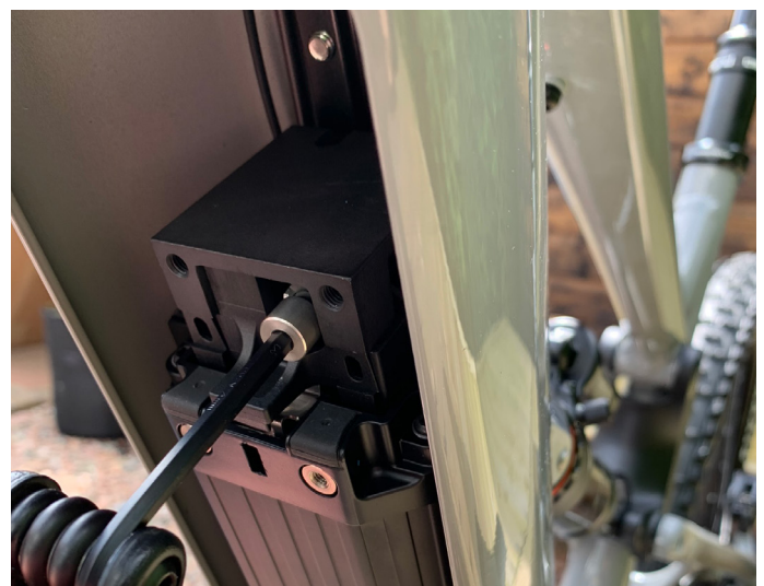
4. Carefully turn the battery release hex clockwise to release the battery. It will slide forward onto a secondary catch which you will need to push down to fully release and remove the battery.
