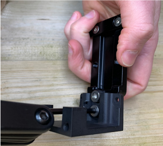
11. Turn the mount 180 degrees and refit on the back plate
