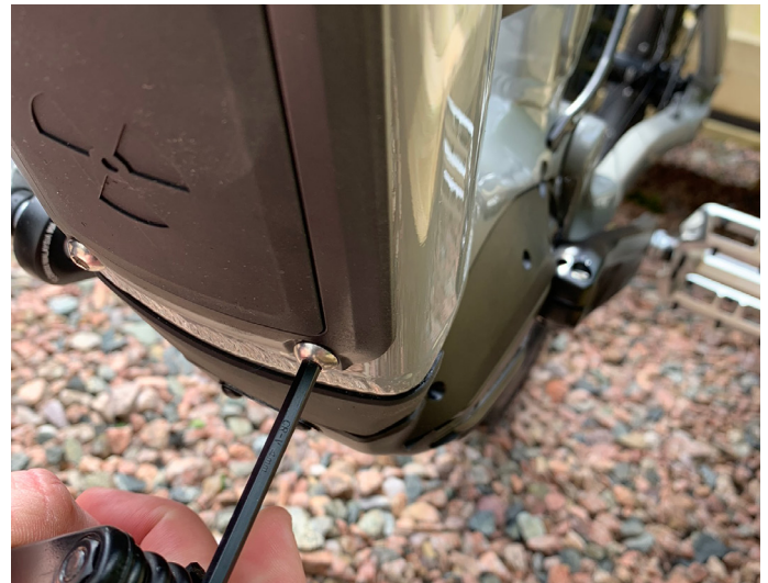
2. Loosen the two bottom bolts 1 full turn
