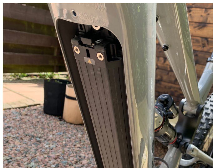
3. Slide battery door upwards to remove
