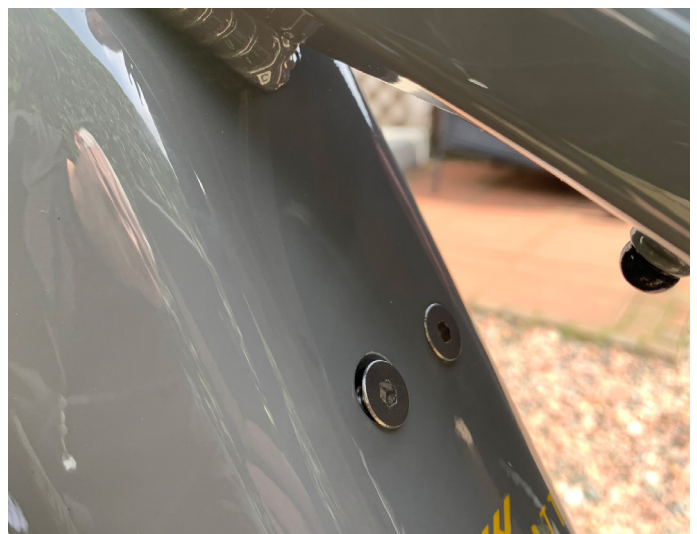
16. Move cables into correct position and then tighten battery mount bolts – be careful not to pinch any cables as you do this
