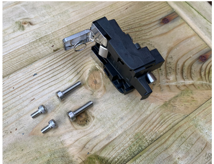
8. Remove this part of the bracket and keep bolts safe
