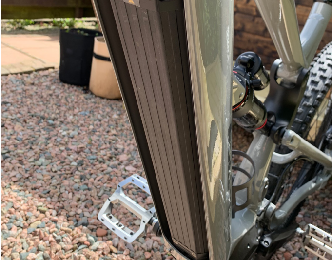
17. Insert the new battery ensuring that the battery is tight in the mount
