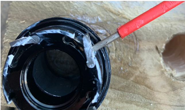
15. Remove the pawls using the flat head screwdriver.
