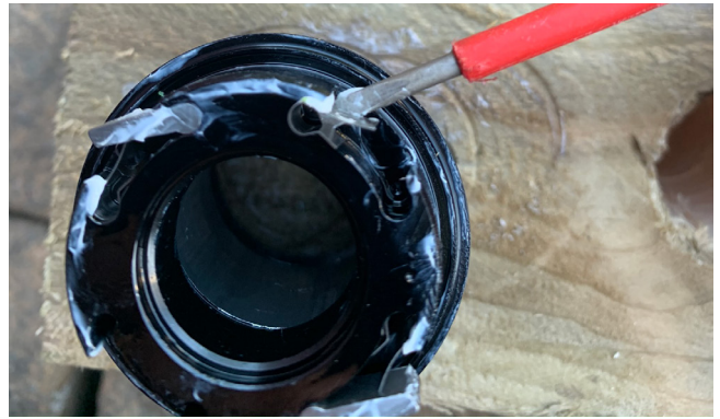
16. Remove the springs using the flat head screwdriver.
