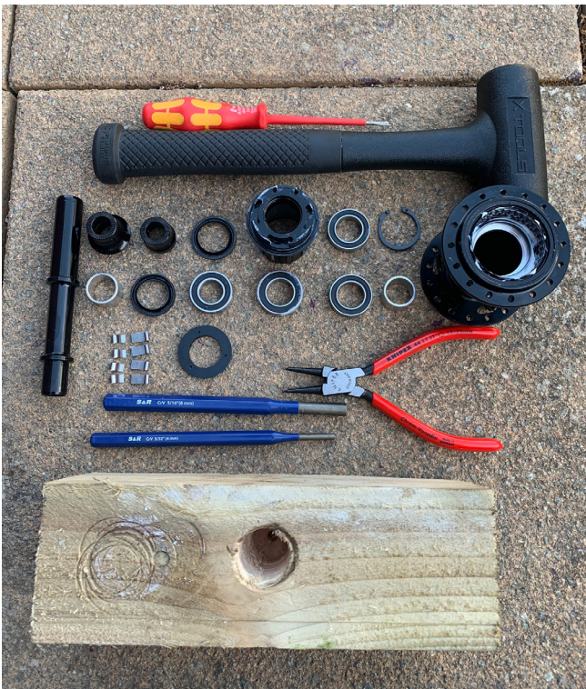
17. The hub is now fully stripped.
