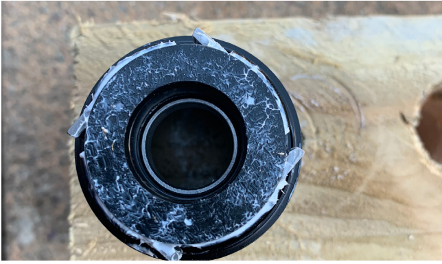
13. Using your bearing punch, hit the last bearing out of the freehub. Again, this bearing should be hit in various places to ensure it comes out straight.
