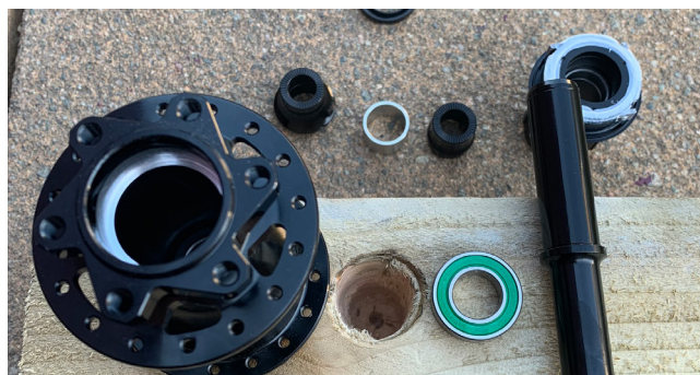
6. Put your hub over the hub support non-driveside down. Carefully hit the end of the axle to remove the non-driveside bearing.
