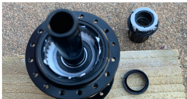
5. Remove seals from hub shell driveside and non-driveside using a flat head screwdriver to lever under the seal.
