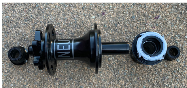
3. Pull off freehub turning the freehub anti-clockwise as you pull.
