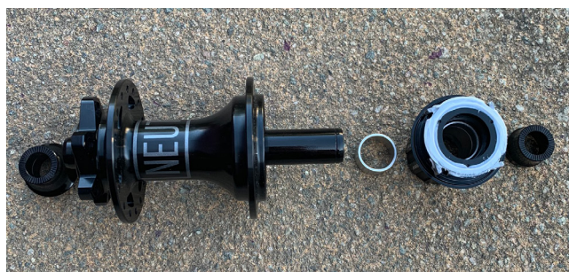
4. Take bushing off the axle (it may be in the back of the freehub).
