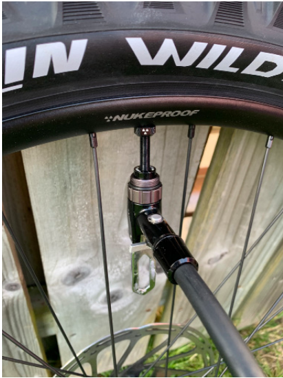
15. Connect your tubeless pump to the valve.
