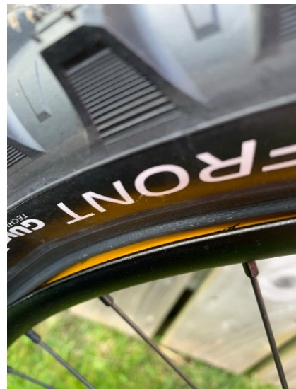
14. Finish fitting tyre. Make sure the bead is pushed to the centre of the rim as this will make it much easier.
