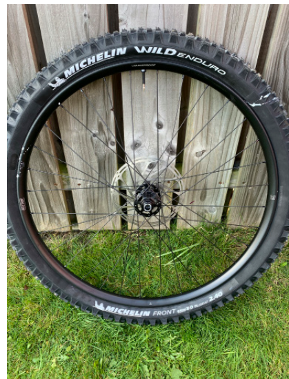
19. Lift your wheel and shake it to get the sealant all round the tyre.
