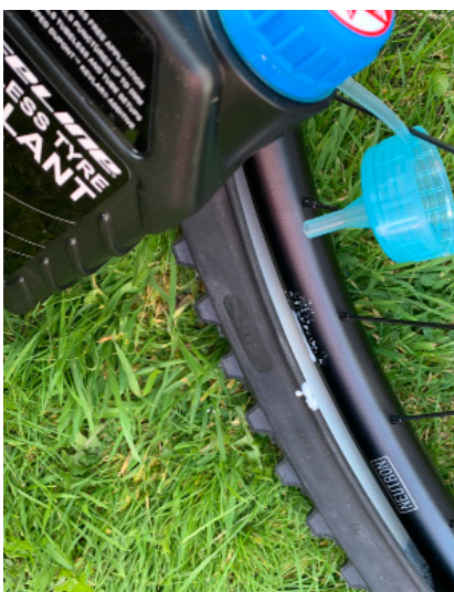
13. Add tubeless sealant as per sealant manufacturer recommended amount.
