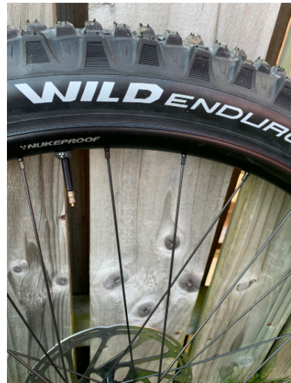
12. Start to refit the tyre, leave ¼ open.
