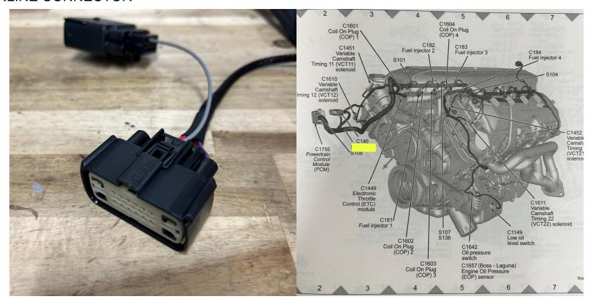
THIS IS THE ACCELERATOR PEDAL CONNECTOR THAT CONNECTS UNDER THE DASH, SUGGEST TO ROUTE THROUGH DRIVER SIDE GROMMET
