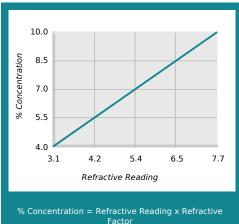
Coolant Refractometer Factor % Brix = 1.3
