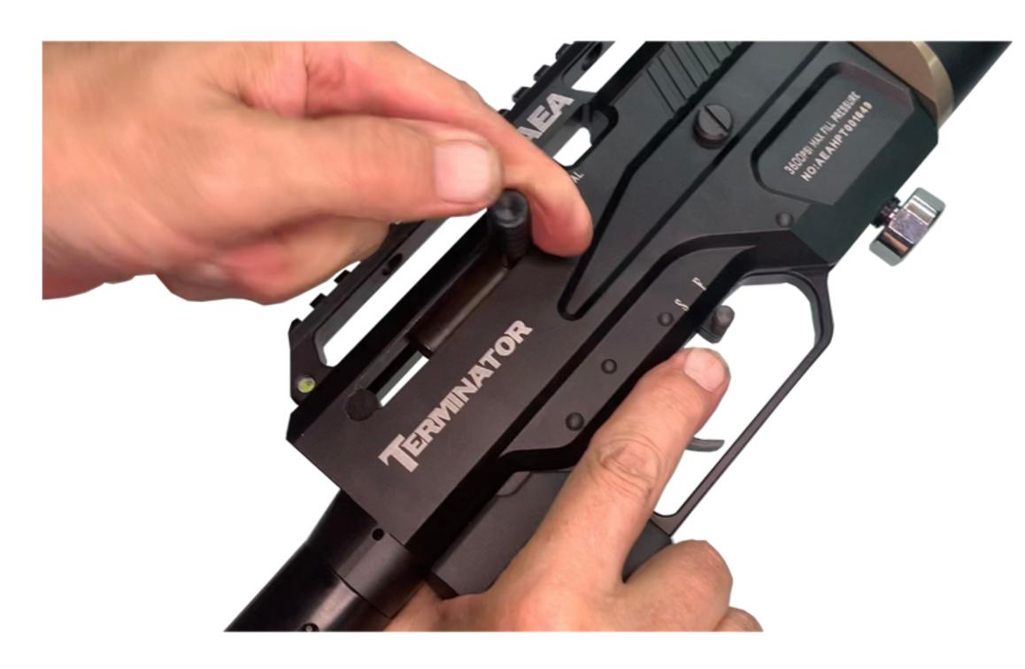
To de cock the hammer, pull and hold bolt handle, remove the magazine from the slot, squeeze the trigger slowly to decock the hammer spring while holding the cocking handle.
