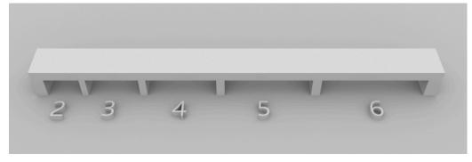
Minimum Hole Diameter and Engraved Detail Width, Z-Axis, at 0.05mm Layer Height
