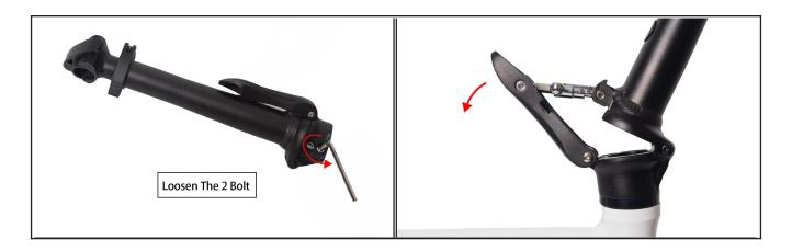
Method: There is a small spherical handle on the side of the handle, pull it to the top, and then pull the handle outward. Fold the stem, and place the plastic cover into it. Tighten the screws, and restore the stem to its original state.
