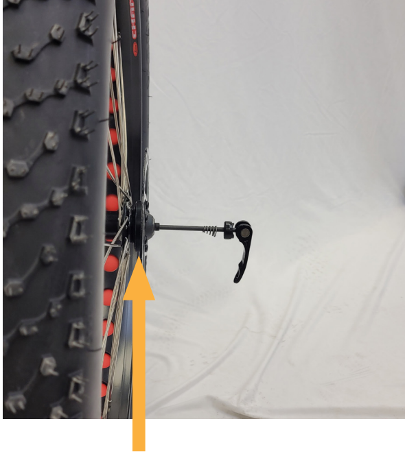
Smaller side of spring to be facing the wheel.
