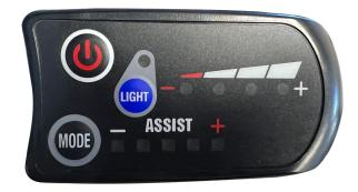
**ON/OFF:** Turn on the power, press the "ON/OFF" button, the power will be turned ON or OFF.
