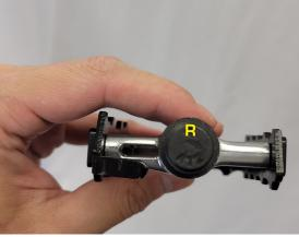
The left pedal is attached by turning it counter clockwise and the right pedal is tightened by turning it clockwise. Make sure the pedals are tightly attached to the crank arms to prevent stripping. (See picture below)
