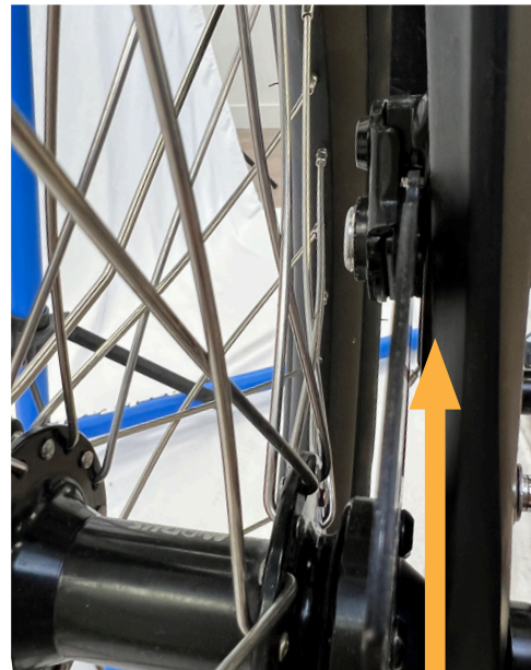
Ensure brake disk and brake caliper are aligned.
