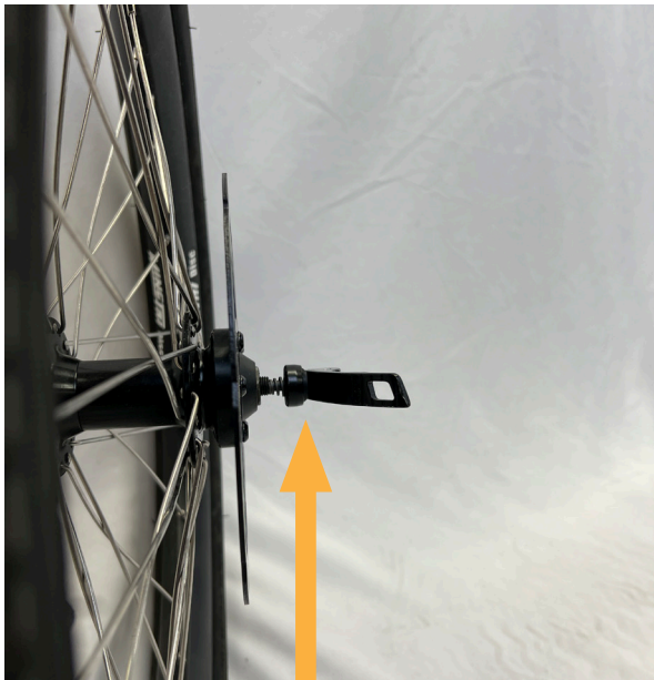
Quick release handle on the caliper side of the wheel.
