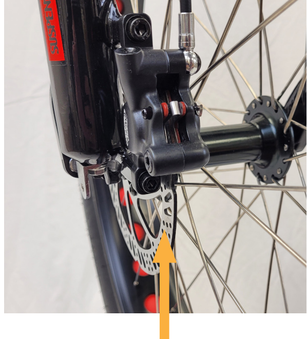
Ensure brake disk and brake caliper are aligned.
