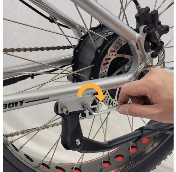
Turn bolts clock-wise to tighten.
