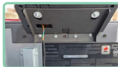
Control Panel Mounting
