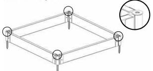
**STEP 3**: Insert widest end of the pole into recess of staking joint stakes – repeat with remaining poles.
