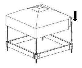
**STEP 2**: Insert support pole into canopy connector cap (*refer to image on left*). *Repeat with remaining poles*.
