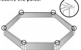
**STEP 3**: Insert widest end of the pole into recess of staking joint stakes – repeat with remaining poles.
