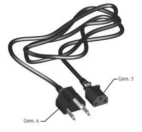
6a.5 Plug Conn. 3 into the control box installed in step 6 6a.6 Plug Conn. 4 into any receptacle on Y1425
