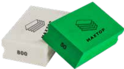
Maxtop Electroplated Diamond Hand Pads 50 grit coarse pad and 800 grit finishing pad. For sanding quartz edge after sawing or routing process and creating a bevel. Located under flap inside installation kit box
