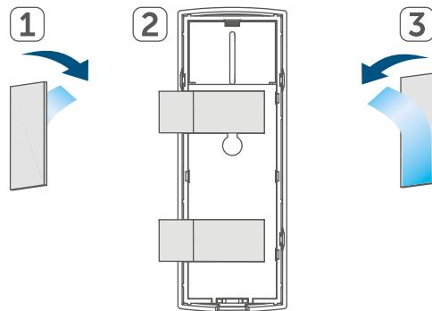
Press the device rear side first onto the chosen position.
