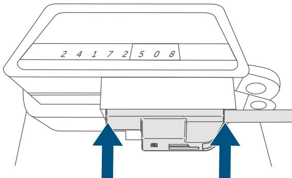
Finally, insert the sensor connector (H) on the underside of the HmIP-ESI into the connection port (E), until it audibly clicks into place (*→see illustration*).
