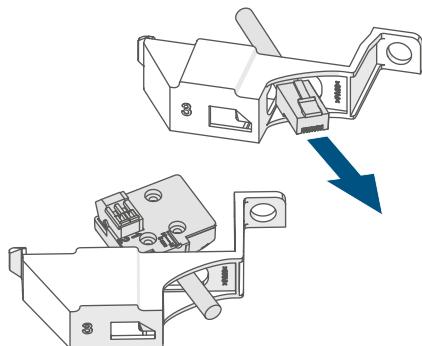
Insert the ES-GAS-2 electronics unit (G) so the guide ribs fit precisely in the guide rails of the adapter:
