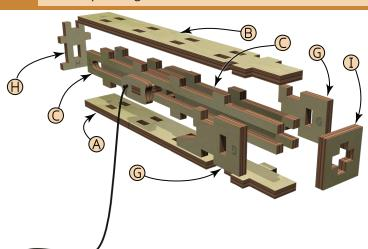
Glue two Sides (C) to the Bottom (A) and Top (B). Slip the nock assembly into the slot, then glue the two Cheek Pieces (G), Muzzle (I), and End Cap (H) into place.
