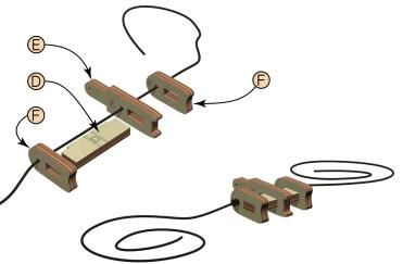
Glue the Nock (E) to the center of the Cross Piece (D) and the Guides (F) to the ends. Thread a piece of cord 2 through the holes leaving an equal amount on both sides. Tie a knot against the outer faces as shown.
