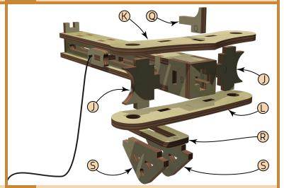
Glue the Braces (J) to the sides of the barrel, then glue the Sight (Q), Upper Frame (K) and Lower Frame (L) in place. Glue together the two Pivot Plates (S) and the Base Plate (R), then glue them to the underside.
