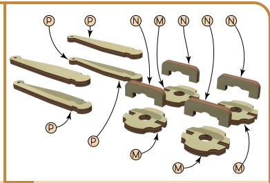
Glue together the Throwing Arm Halves (P) to create two throwing arms. Glue a Winder Bar (N) to each of the Winder Plates (M).
