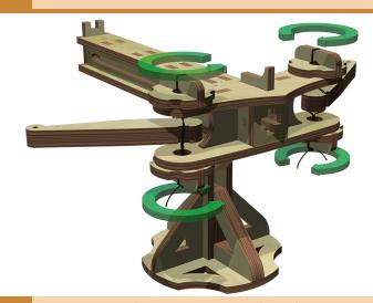
Repeat step 7 for the other side. "Sieze" the knots with a drop of glue and trim any excess cord. Rotate each winder one half turn as shown.
