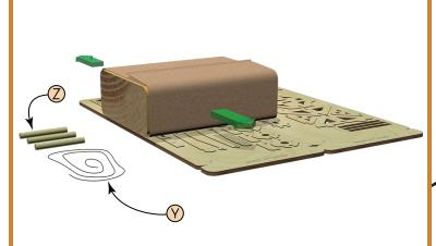
Remove and set aside the Cord (Y) and the Ammo (Z). Sand both sides of the carrier boards first with 150 1 grit and then 220 grit sandpaper. Cut the Cord (Y) into three equal lengths.
