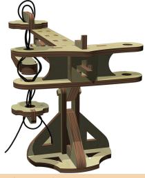
Use a cord (the skein) to make two loops around the winders and throwing arm, passing through the holes in the frames. Pull the ends tight, and tie a double knot over the lower winder bar.
