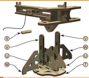
Glue together the two Center Frames (U), two Uprights (V), two Outer Frames (W), and the Base (T). Slip the Pivot Pin (X) through the Uprights (V) and pivot. Fix it with a drop of glue.
