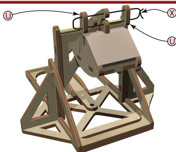
**8** Thread Cord (X) through the Link Plates (U), throwing arm, and counterweight as shown. Knot the cord tightly against the link plate, and "sieze" the knot with a drop of glue. Trim any extra cord with scissors.
