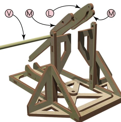
**5** Glue the Cheek Pieces (M) to the Throwing Arm (L), ensuring the holes are aligned. Slide the Axle (V) through the uprights and throwing arm. Glue the axle to the gantry braces.
