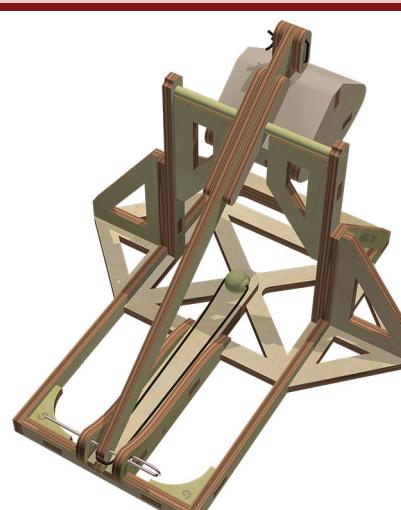
**10** Load the ammo as shown and use a straightened paper clip for the trigger.
