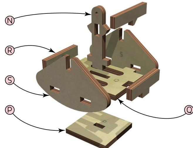
**6** Glue the Counterweight Bar (N) to the Base Plate (P) and Floor (Q). Glue the End Frames (R) and Cross Bar (T) in place. Glue the Side Frames (S) to the assembly.
