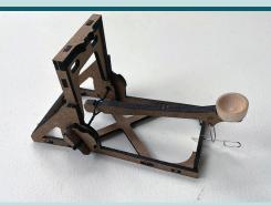
Lower the arm and slip the trigger pin through the trigger and into the hole in part 'F'. Voila!
