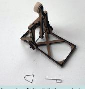
Bend both ends of the 'U' shaped piece inwards. (Roughly  $1/8^{\prime\prime}$  or 3mm)
