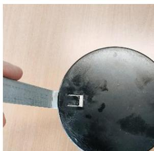
Attach the plug pins to the floats
