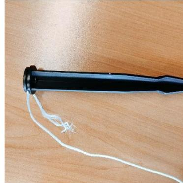
Attach the nylon rope to the anchor pin at the desired length
