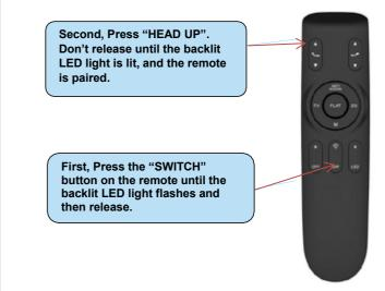
When Pairing Program Button on the control box and the backlight LED on the remote stop flashing, and the buzzer on the control box has a "DI" sound, pairing is completed. If the pairing fails, repeat the process again.
