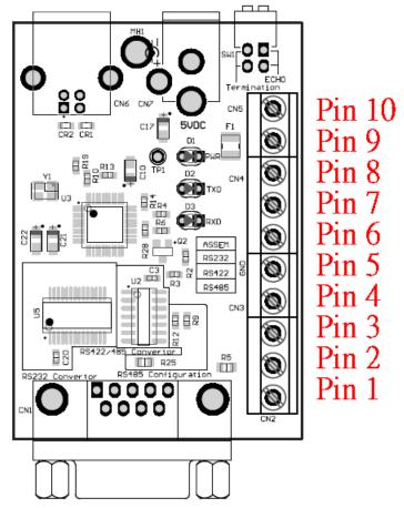
Figure 2.1 - USB2-H-1001-M Terminal Block Connector Assignment
