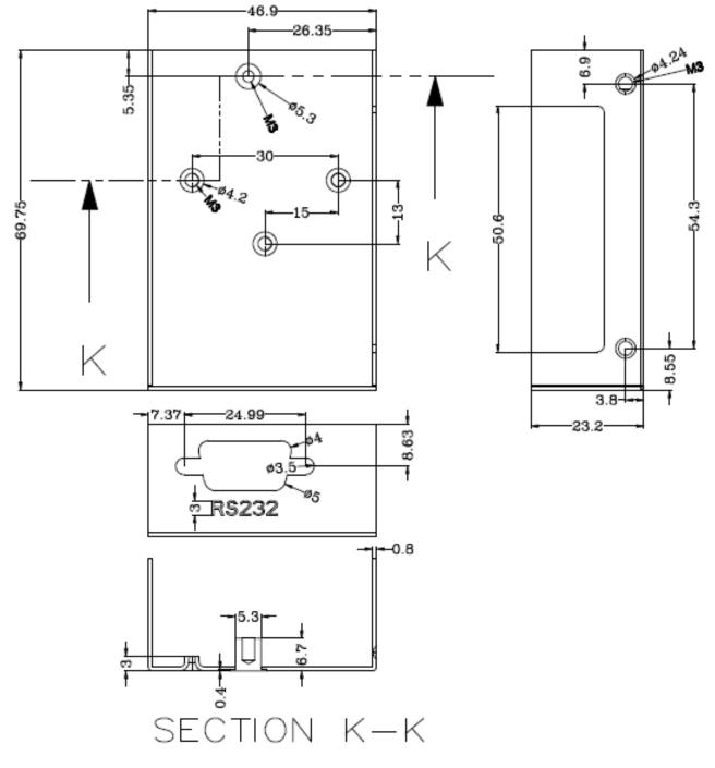
Figure 5.2 - USB2-H-1001-M Bottom Cover Dimensions
