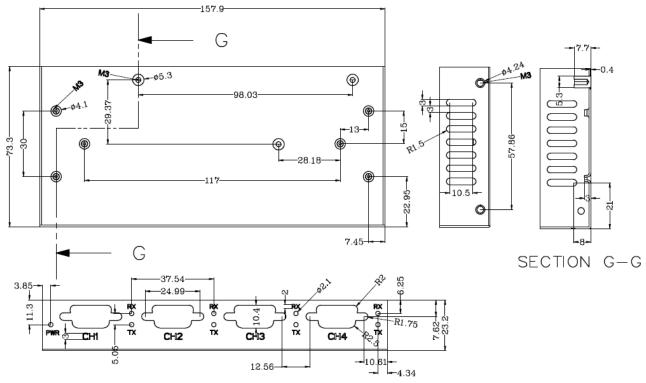
Figure 5.6 - USB2-H-1004-M Bottom Cover Dimensions
