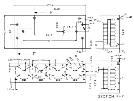
Figure 5.8 - USB2-H-1008-M Bottom Cover Dimensions
