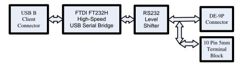
Figure 1.4 - USB2-H-1001-M Block Diagram
