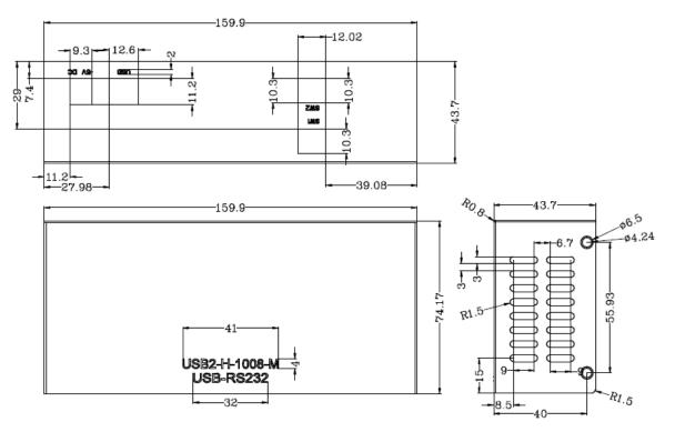
Figure 5.7 - USB2-H-1008-M Top Cover Dimensions
