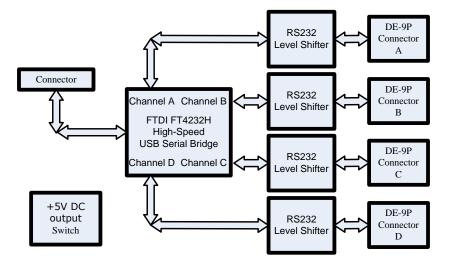
Figure 1.7 - USB2-H-1008/1016-M Daughter Board Block Diagram
