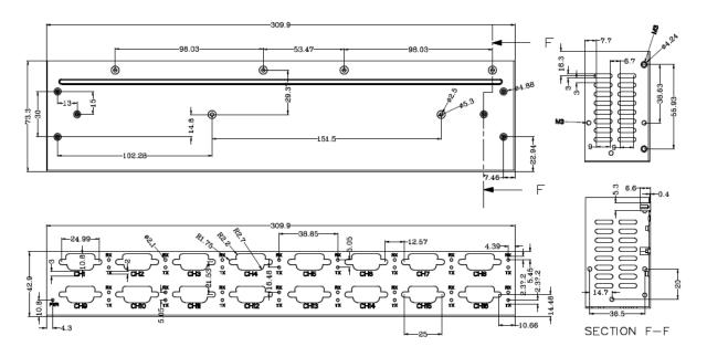
Figure 5.10 - USB2-H-1016-M Bottom Cover Dimensions
