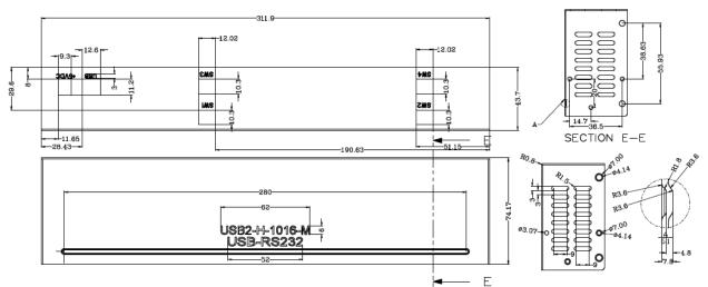
Figure 5.9 - USB2-H-1016-M Top Cover Dimensions
