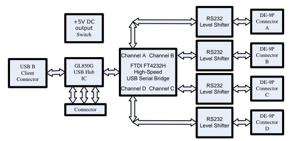
Figure 1.6 - USB2-H-1004/1008/1016-M Main Board Block Diagram
