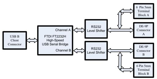
Figure 1.5 - USB2-H-1002-M Block Diagram
