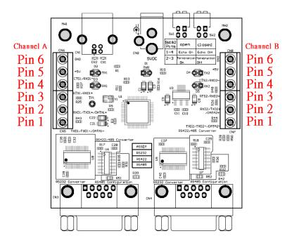
Figure 2.2 - USB2-H-1002-M Terminal Block Connector Assignment
