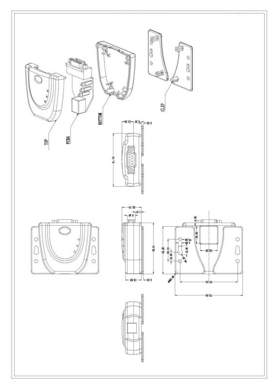
Figure 4.2 - USB2-F-6001 Case Dimensions with UniClip
