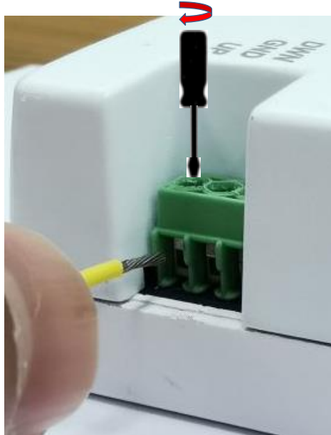
Figure 7 - Clamping wire with screwdriver in clockwise direction
