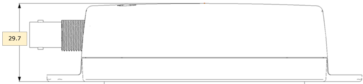
Figure 6 – LDSBus EC Sensor Adapter Dimension – Side View
