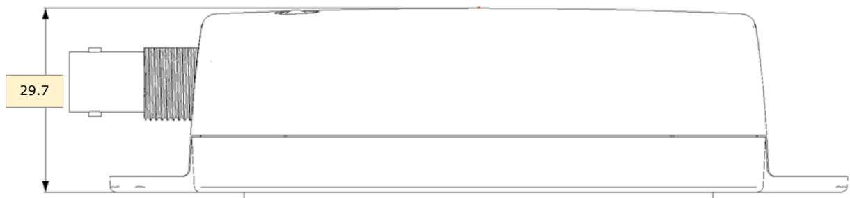
Figure 6 – LDSBus Dissolved Oxygen Sensor Adapter Dimension – Side View
