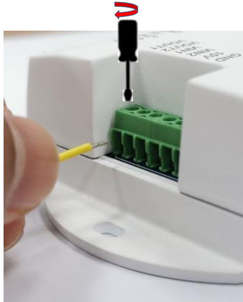
Figure 5 - Clamping wire with screwdriver in clockwise direction
