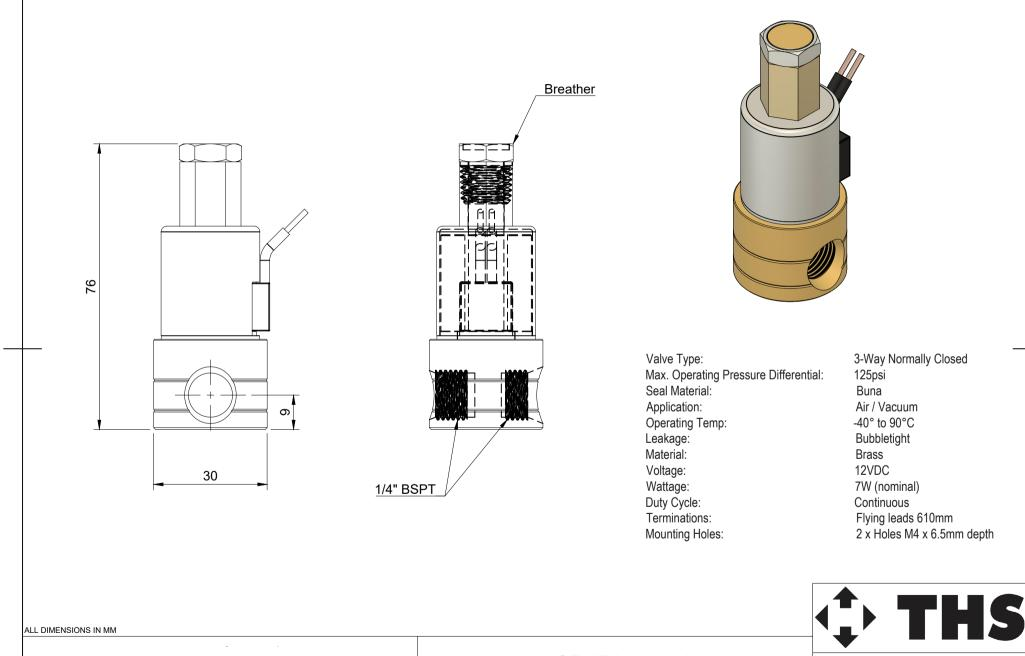
12V NC Air / Vacuum Solenoid Valve For Eletctric/Air Systems
