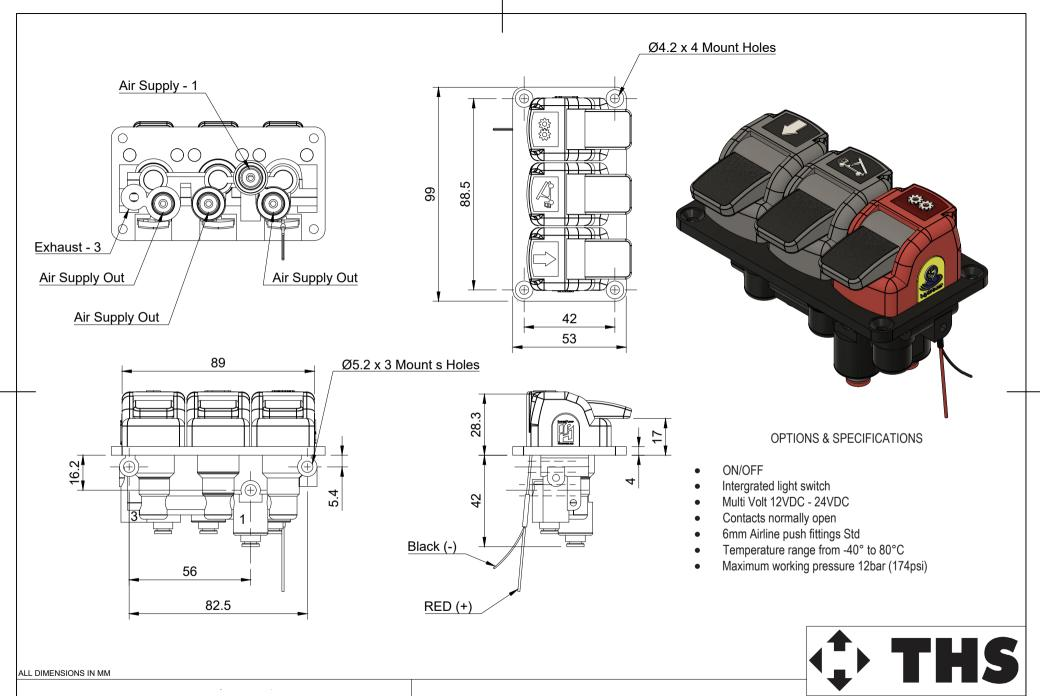
On/Off Cab Switches For Air Systems
