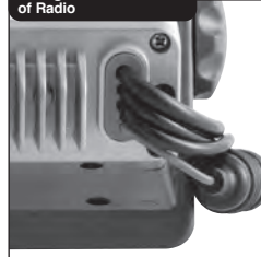
Wiring Located at Back of Radio
