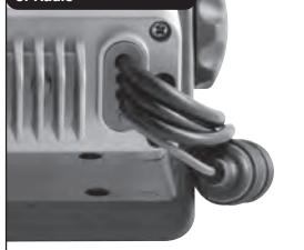
Wiring Located at Back of Radio
