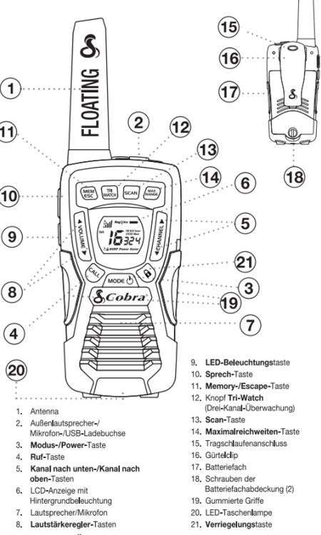
**FUNKSPRECHGERÄT, MODELL AM1055 FLT**
