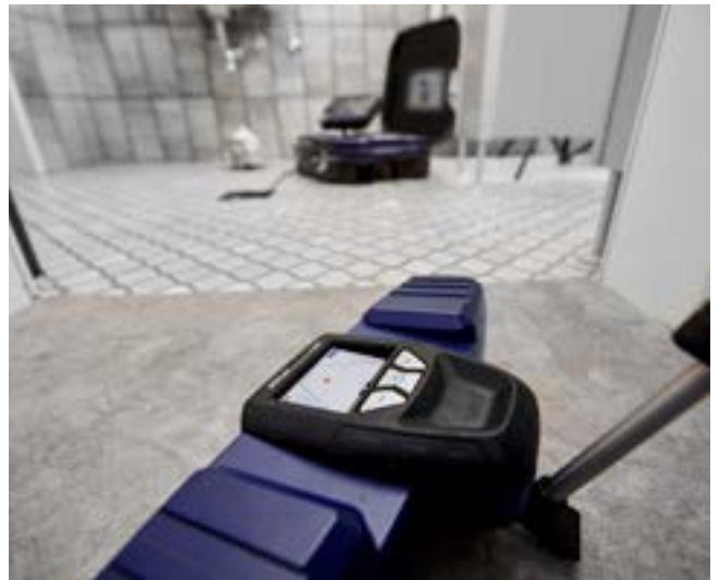
Precise location of the camera head with the Wöhler L 200 Locator
