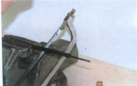
2: Cut the damaged outer shaft
