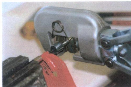
10: Press 3 times with the press tool (16 kvadrat)
