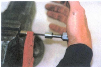
8: Attach the new brush connection
