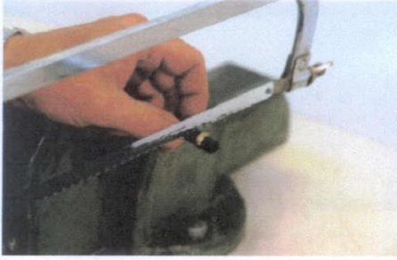
3: Cut the damaged outer shaft
