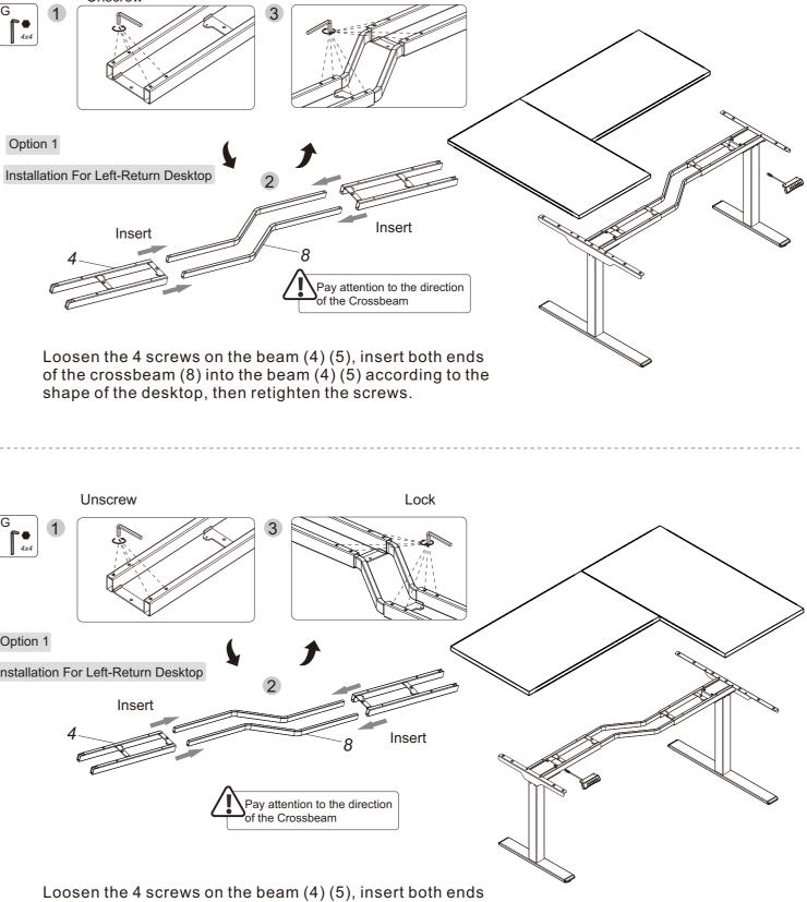
of the crossbeam (8) into the beam (4) (5) according to the shape of the desktop, then retighten the screws.
