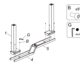
Use screws (B) to connect the table legs (1) with the support beams (4) (5), and tighten them with a wrench (G).
