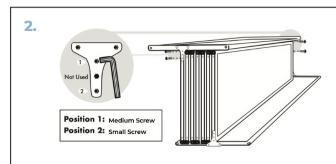
Line up bracket on end panel to the holes on the outside piece of panel bundle. Screw two bolts into each bracket on the end of the panels as shown.
