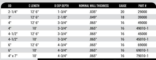
Our standard stock is in 10′ and 12′6″ lengths, but we will cut to your specifications ∗ID of Expansion = Tube OD
