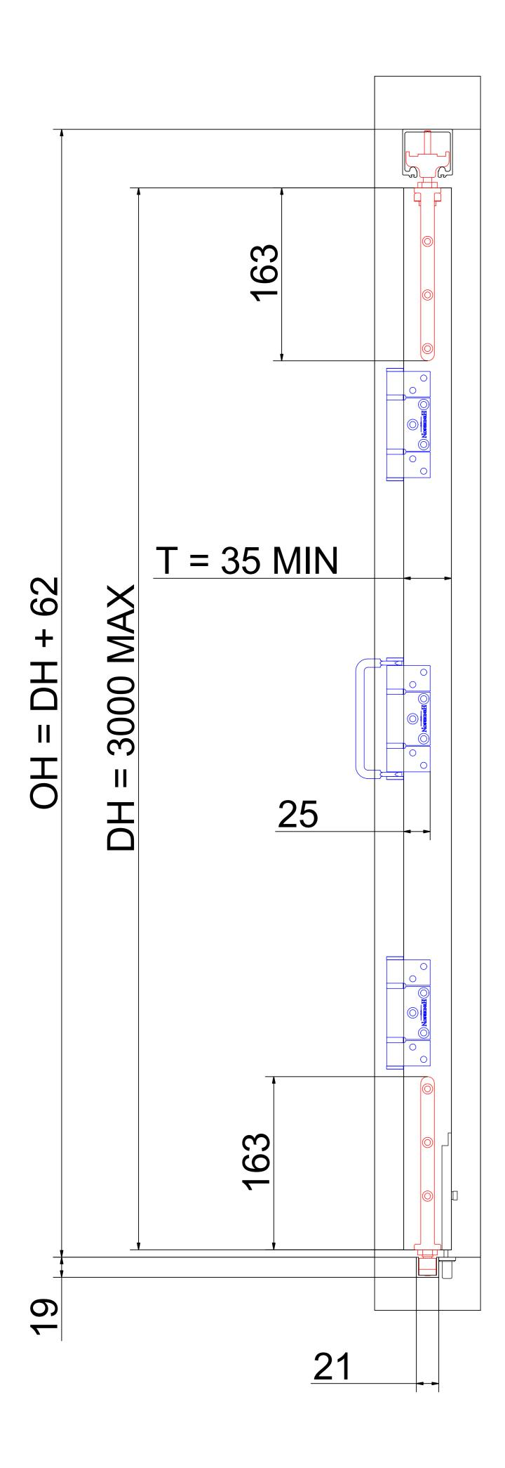
NOTES: 1. DRAWING IS FOR REFERENCE AND SUBJECT TO CHANGE WITHOUT NOTICE. 2. APPLICATION IS FOR INTERNAL TIMBER DOORS WEIGHT MAX 45KG. REFER TO FITTING INSTRUCTIONS FOR ROUTING DETAILS REQUIRED 3. 110mm FLUSHBOLTS SHOWN. ALTERNATIVE SIZES ARE AVAILABLE. 4. FOR DOORS LESS THAN 45mm THICK ALTERNATIVE FLUSHBOLTS ARE REQUIRED. 5. 6. ALL DIMENSIONS ARE IN MILLIMETERS
