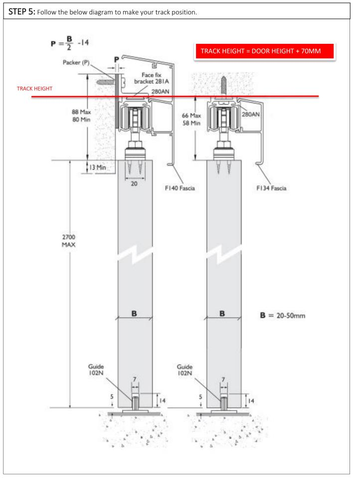
**STEP 6:** Fix track into position using preferred fixing methods (face fixed or soffit fixed) following measurements from step 5.
