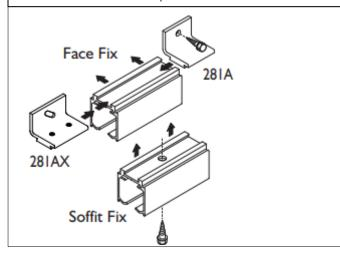
**STEP 8:** Based on your desired layout. Secure the track into position.
