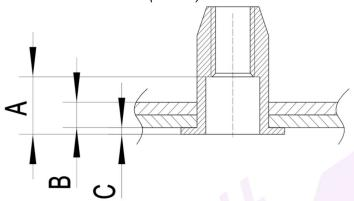
A = depth of the rivnut (inside of the rivnut non-threaded and no upset part of the rivnut when setting);
