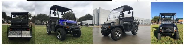
The Taurus 200 GV is equipped with a 9.5 HP air and oil cooled high performance 177cc GY6 engine with internal reverse set up. It comes standard with a H/L gear. The low gear mode has a 40% better climbing ability than the non H/L version and can climb up to 30 degree slopes with ease. The Taurus 200 has significantly greater torque than the non H/L gear version machines. It is also equipped with 4 wheel independent suspension for optimal driving experience.
