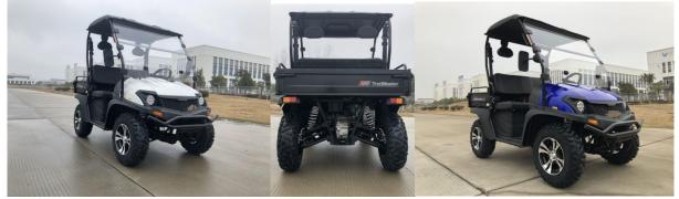
Other notable features includes: aluminum wheels package, large and aggressive front and rear 24 x 8-12 / 24 x 8-12 off-road tires, Hi/Lo LED headlights, turn signals, rearview side mirrors, digital dashboard, hard top, steel front bumper, retractable seatbelt, 12 volt outlet, cup holder.
