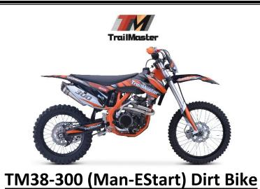
The TM 38-300 is a great full size dirt bike. It is has both a kick start and a new "ELECTRIC START". It has a high performance liquid cooled 298cc 4 stroke 31hp engine with kick start and a top speed of around 65 MPH and a seat height of 37". It is available in red, green, and orange colors. The TM38 features a 6 speed manual transmission with front and rear disc brakes, inverted front shock, and a lightweight steel tube frame! This is sure to be a HOT seller!
