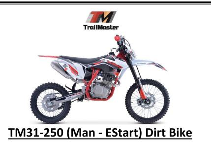
The TM 31-250 is a great full size dirt bike. It is has both a kick start and a new "ELECTRIC START". It has a high performance 223cc 4 stroke 16hp engine with kick start and a top speed of around 55 MPH and a seat height of 34.6". It is available in red, green, and orange colors. The TM31 features a 5 speed manual transmission with front and rear disc brakes, inverted front shock, and a lightweight steel tube frame! This is sure to be a HOT seller!
