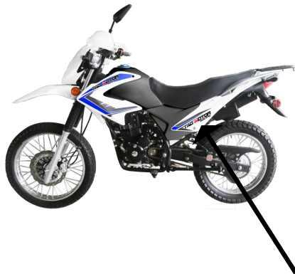
Main Fuse Location
