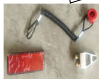
Rear reflector Brake lever tip(you may find it already assembled to the brake lever) Safety kill switch cable
